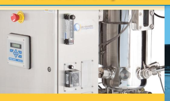
The EVO series of sterilizable-in-place (SIP) fermentors and bioreactors are easy-to-use customizable culture systems. Each EVO unit is equipped with a non-proprietary integrated control system that is common to the entire range of DCI-Biolafitte fermentors and bioreactors, offering a scalable solution from research and development through production.
